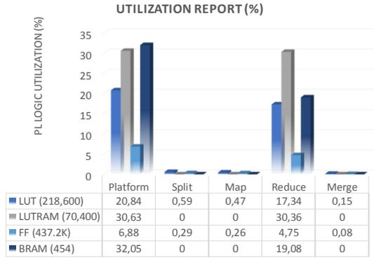
Figure III. Hardware platform utilization report.
