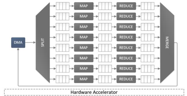
Figure I. Hardware accelerator architecture. The DMA is managed by the systems PS' and sends and recovers data from the hardware accelerator.
