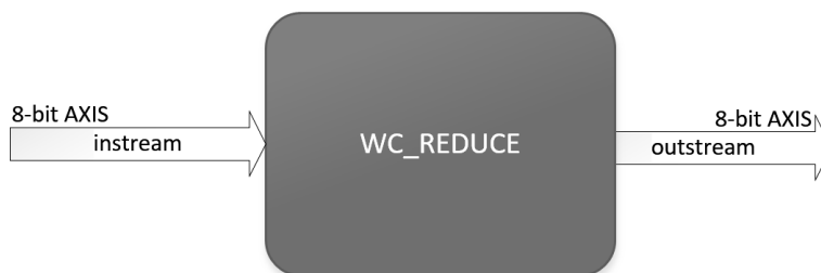
Figure 35. - Reduce IP block
