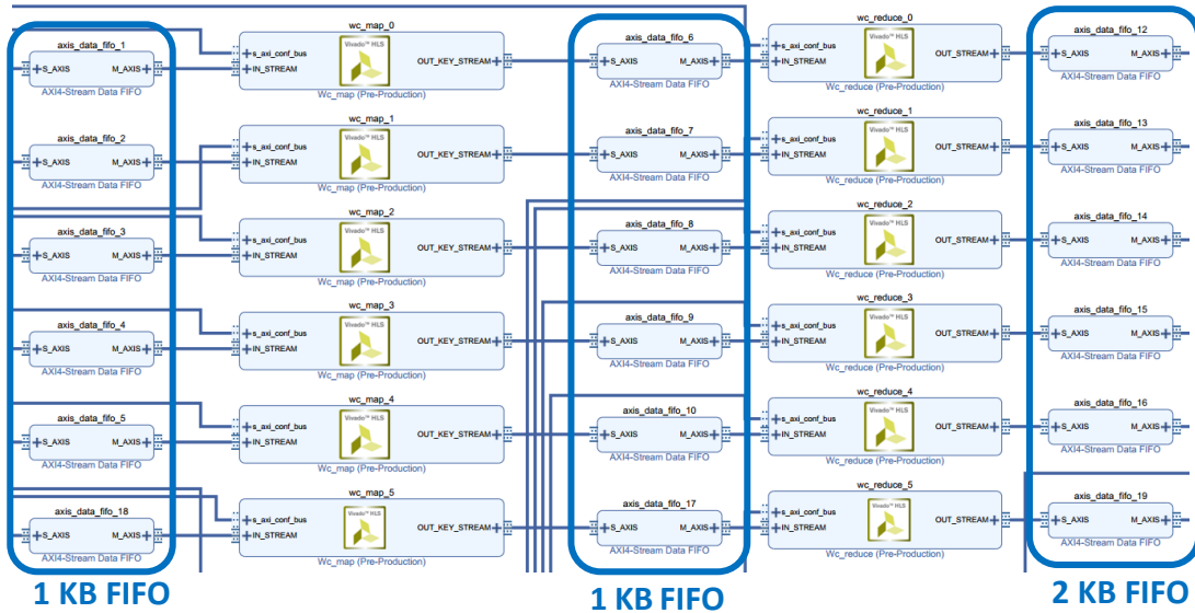
Figure 41. - FIFO position and configuration
